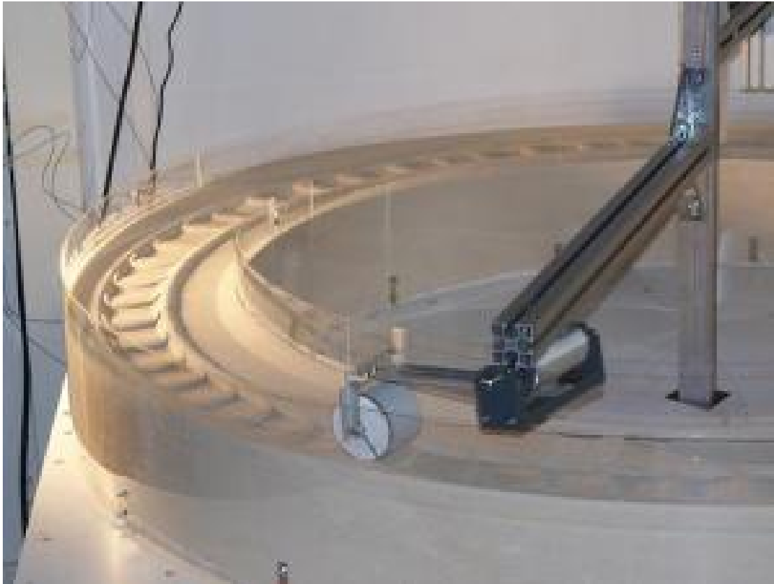
Lyon washboard road experiment, featuring a wheel rolling over a bed of sand, creating ripples. (Credit: Stephen Morris)
